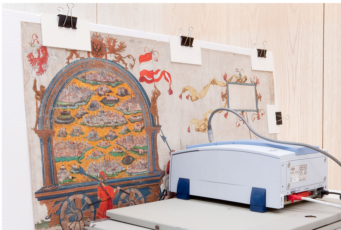
Fig. 2: FTIR analysis of the pigments used for a medieval miniature painting on parchment
